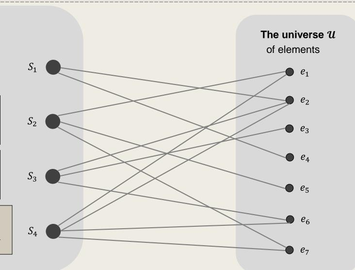
Pick a minimum cost vertex subset from the left, such that every vertex on the right is adjacent to at least one chosen vertex on the left.
