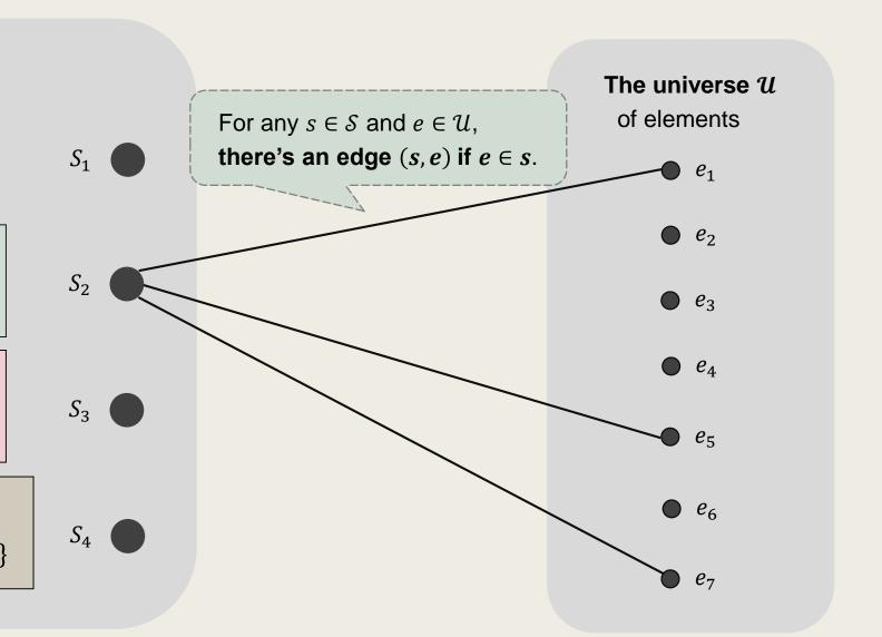
Pick a minimum cost vertex subset from the left, such that every vertex on the right is adjacent to at least one chosen vertex on the left.
