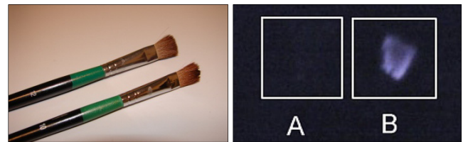
Figure 2. Left: dry brush A (12mm) and wet brush B (10mm) Right: the corresponding IR footprints.
