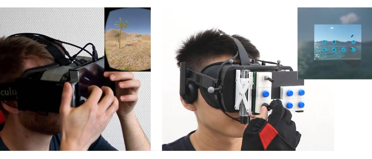
FaceWidgets enables tangible interactions using **physical controls on the HMD backside**
