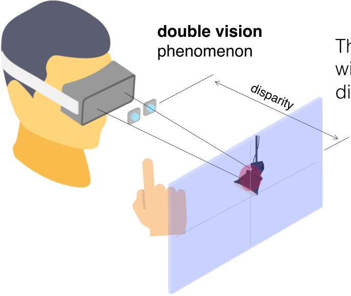
The button out of fixation point will be seen as double at near distance, called **double vision**.
