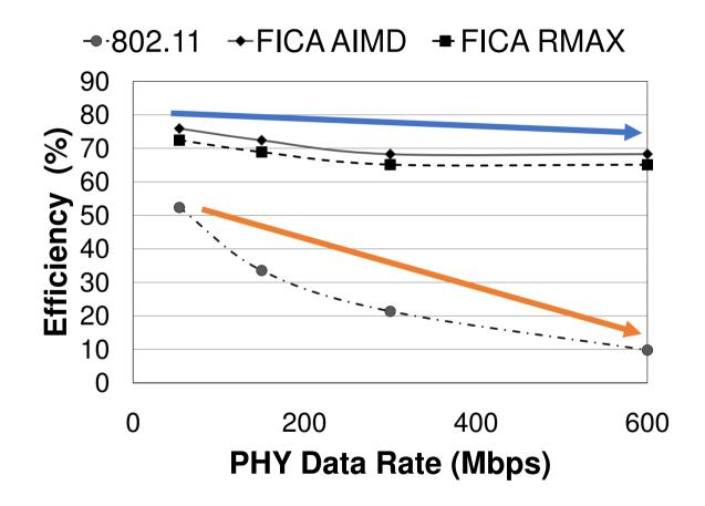
Efficiency is nearly stable when the PHY data rate increases
