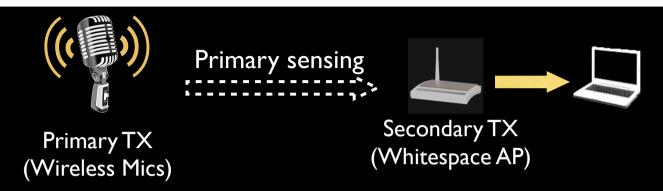
Secondary transmitters should sense for primary transmissions before channel use
