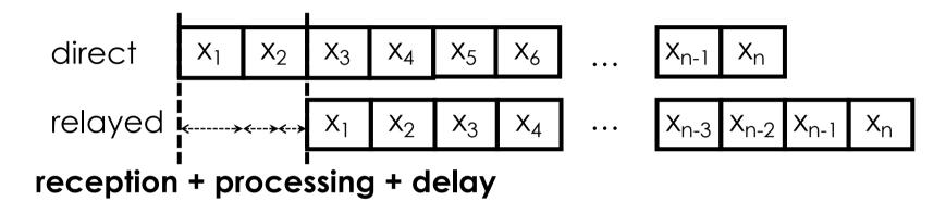
Structure of combined signals is analogous to convolutional code
