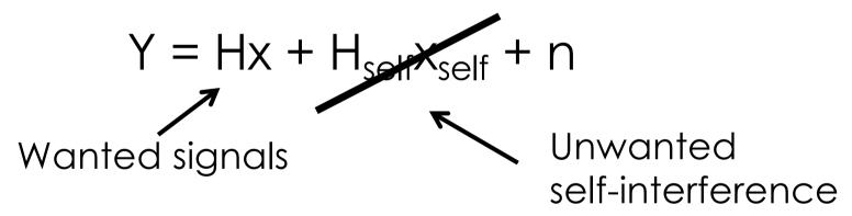
Challenge 1: self-interference is much stronger than wanted signals, i.e.,  $|H_{self}|^2 \gg |H|^2$
