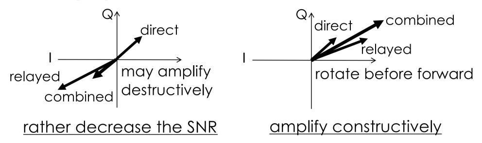
2. Demodulate-and-forward [DelayForward, MobiHoc'16]
