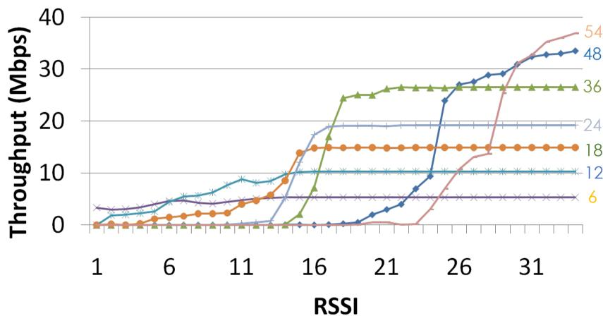
throughput =  $(1-PER_{r,SNR}) * r = (1-BER_{r,SNR})^N * r$  $r^* = arg max throughput_r$
