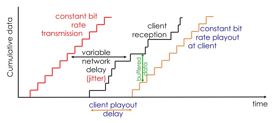
End-to-end delays of two consecutive packets: difference can be more or less than 20 msec (transmission time difference)
