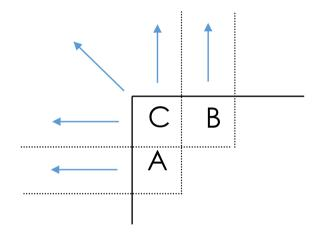
Extended motion vector range from [-16, 15.5] to [-31.5, 31.5], with the following restrictions, depending on its predictor (P):
