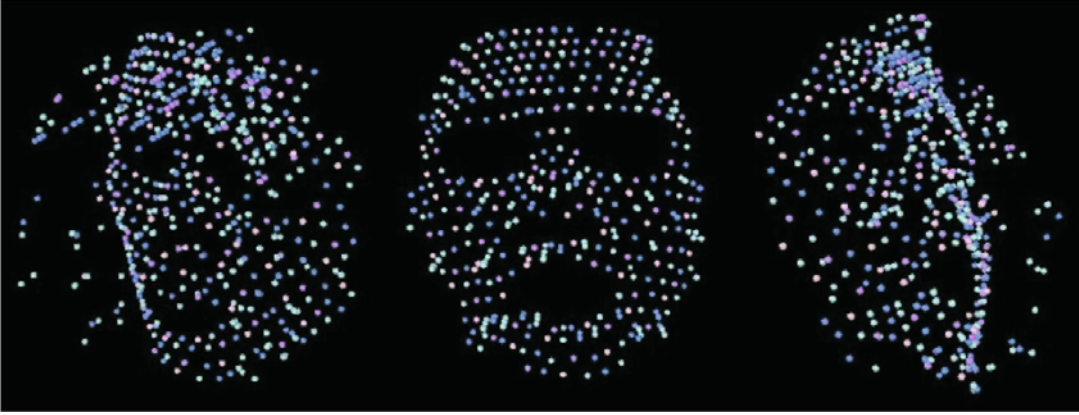
Fig. 8. Potential 3D candidates generated under the mirrored epipolar constraint and the distance constraint. 3D candidates are first constructed from candidates of point correspondences; those whose positions are out of a bounding box are removed from the list of potential candidates
