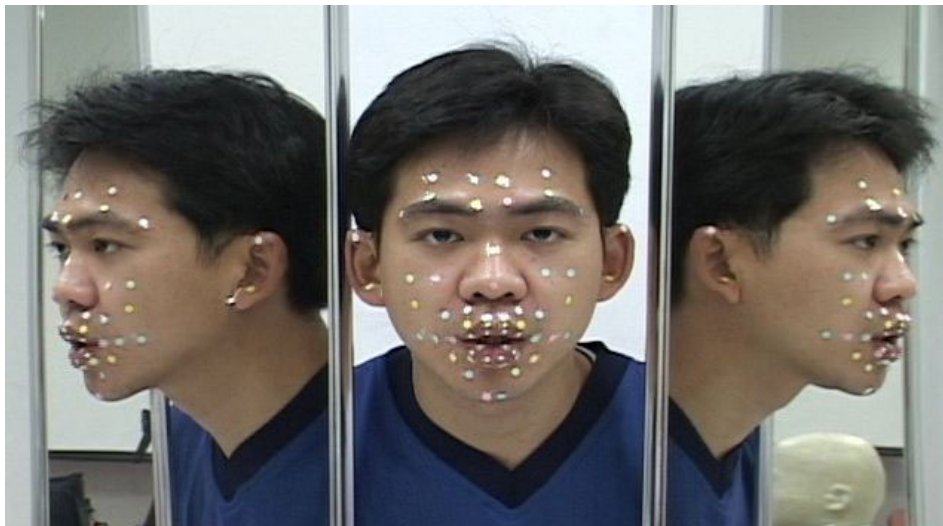
Figure 4.2 A mirror-reflected multi-view video clip captured by a digital video camera in 720×480-pixel resolution. (55 markers: 10 for the lip contour, 12 for lip surfaces, 10 for mouths, 8 for cheeks, and 10 for the forehead)
