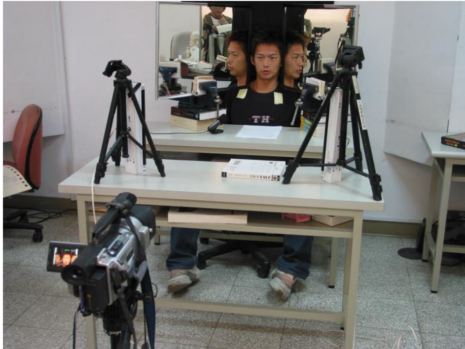
Figure 4.1 Equipment setting. Two plane mirrors are placed near a subject's cheeks and a single video camera is applied to capturing front and side view images simultaneously.
