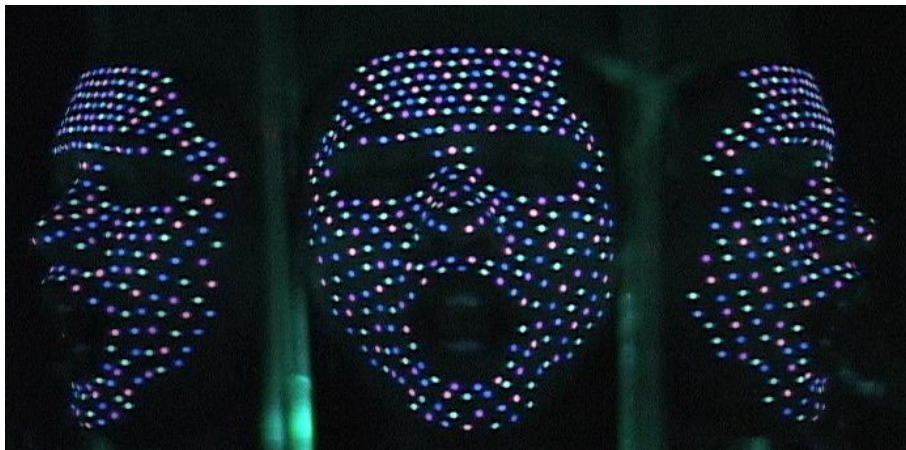
Figure 5.2 A captured video clip of fluorescent markers illuminated only by UV “Blacklight Blue” lamps. The fluorescence is visible in the visible light spectrum and no special lens is required for filtering. (300 markers are evenly pasted upon a subject’s face.)
