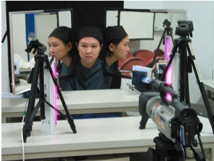
Figure 5.1 The tracking equipment for the blacklight condition. The photo is taken under normal light. Two “Blacklight Blue”(BLB) lamps are placed in front of a subject and mirrors. The low-cost special lamps are coated with fluorescent powders, and it can emit long wave UV-A radiation to excite luminescence.
