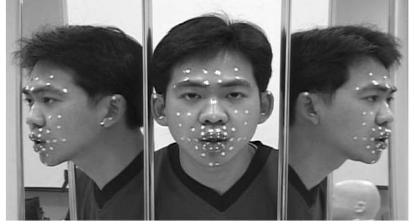
**Figure 3.** The image data captured by DV camera (resolution: 720x480 pixels). 55 markers are placed on the subject's face and lips.
