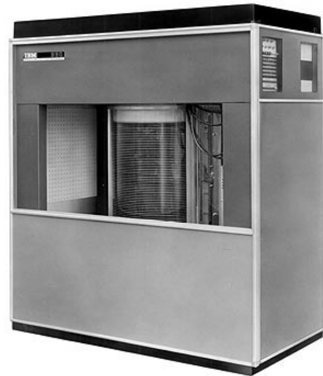
IBM 350 Disk Storage Unit (1200 rpm, 5MB storage)
