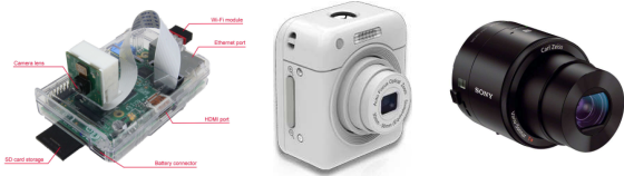
Figure 7: Photos of the considered smart lenses: Smart Beholder (left), Altek Cubic (middle), and Sony QX100 (right).
