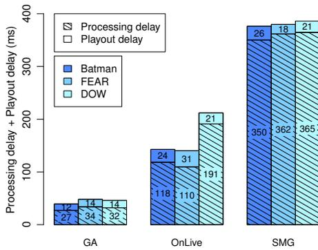
Figure 3: Response delays of GamingAnywhere, compared to two commercial systems, OnLive and StreamMyGame.
