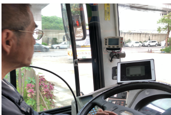
Figure 7: The bus telematics system received a boarding request from the user with a sound notification.
