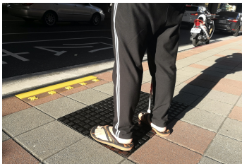
Figure 6: Acrylic prototypes of tactile indicators tested in the field.
