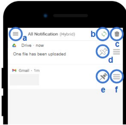
Figure 1. All-notification interface includes: (a) Hamburger menu button for expanding the category menu; (b) Visual indication showing if the notifications are automatically sorted: green indicates sorted and red indicates unsorted; (c) Clear-all-notifications button; (d) Pinning button (before); (e) Pinning button (after); (f) Sorting button
