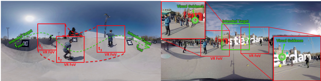
Figure 2 Illustration of two focus assistants on two types of videos: SPORT and TOUR, respectively. All red boxes denote example of a viewer’s Field-of-View (FoV) in VR device. Left-panel: Auto Pilot is applied to help continuously focus on the moving intended target (skateboarder) in the Sport video. We overlaid images of three temporal locations ( t_1 , t_2 , t_3 ) to highlight the motion of the intended target. Right-panel: Visual Guidance (the augmented green arrow) is applied to help refocus on the intended target described in the Tour video. We show two examples of guidance from the left and right towards the intended target in the middle. Note that the guidance dynamically changes according to the spatial relation between a viewer’s head pose and the intended target.
