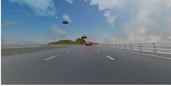
Figure 7: An example eye-movement trace trajectory. The elapsed time between the start of a handover request and when the driver's sight shifted to the obstacle object is termed gaze-shift duration ; the red-marked area is for distinguishing whether the gaze point was on the obstacle.
