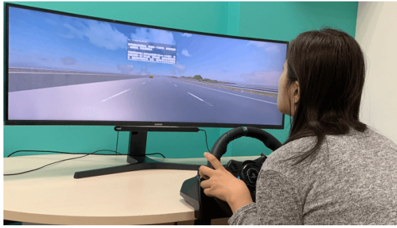
Figure 1: The driving simulator with eye-tracker
