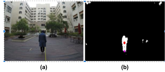
Fig. 7. An example of (a) original image and (b) its segmentation results of human label by FRRN. Red point represents the cluster center estimated by Mean Shift and pink point is the interaction point between the object and the ground plane.
