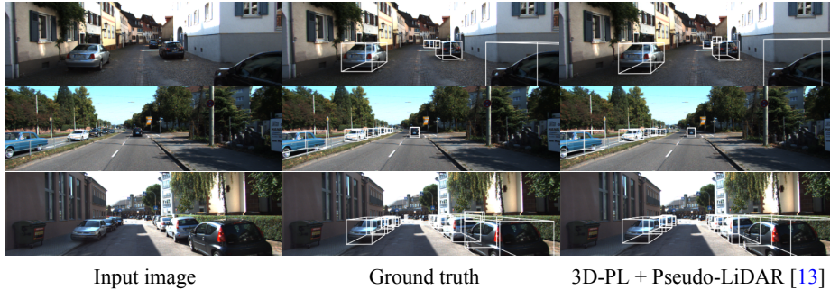
Fig. 1: 3D object detection results using 3D-PL.
