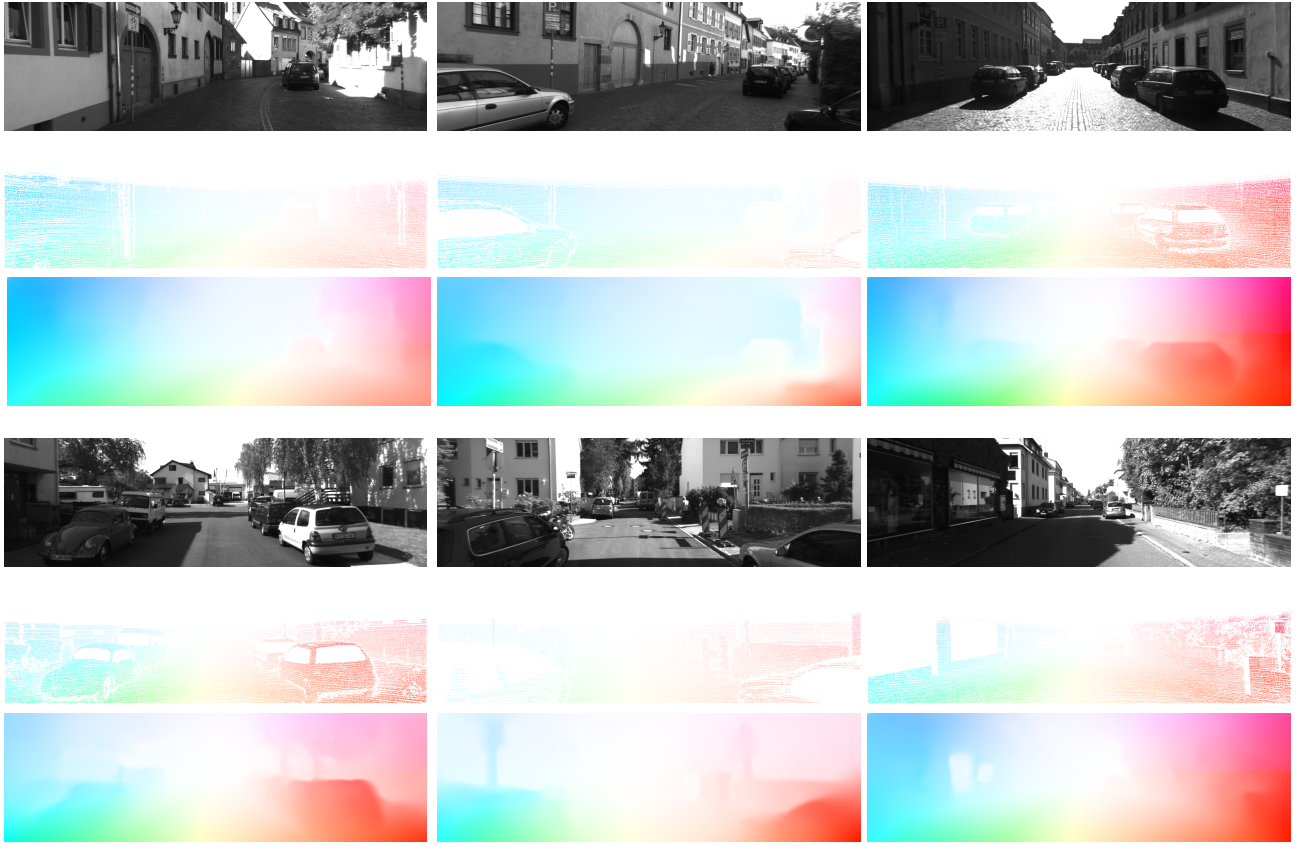
Figure 3: Estimated optical flow results on KITTI 2015. There are 6 examples and from top to bottom, they are real gray-scale images, ground truths and our estimated maps.
