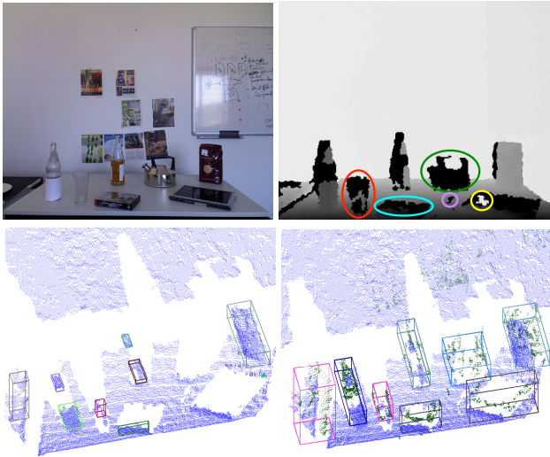
Figure 1: (top) Failure cases of Kinect 3D sensor: (red) transparency, (green) specularity, (cyan) dark objects under flat viewing angle, (yellow) reflections of the projected dot patterns, (violet) interference of dot patterns by reflections. (bottom) We evaluate on a object segmentation task, left: result on Kinect point cloud only, right: strongly improved result on our fused estimate proposed in this paper. (blue points: kinect; green points: cross-modal stereo)
