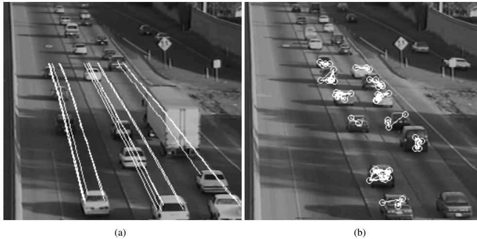
Figure 1.5: Results of Beymer's system [15]. (a) Sample feature tracks. (b) Sample feature groups.
