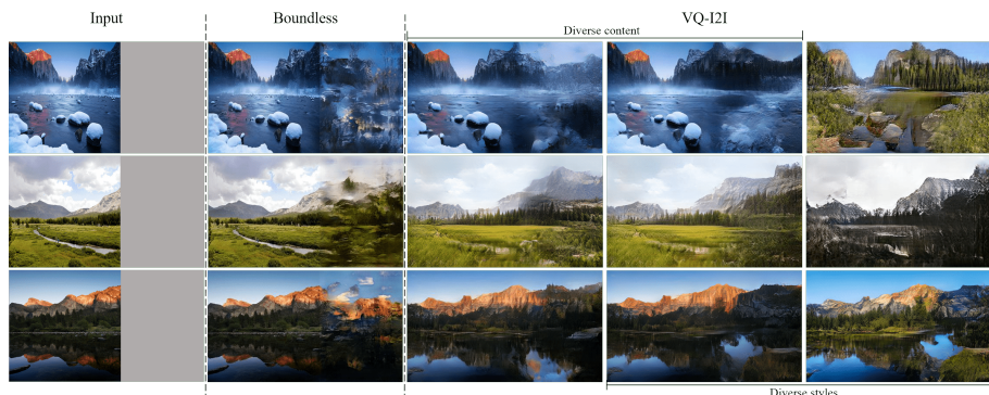
Fig. 5. Qualitative Examples on Image Extension. Example results of image extension on Yosemite [34] datasets, where the comparison with respect to Boundless [31] baseline is also provided. The leftmost column shows the input images for the image extension, where the model takes left portion of size 256 \times 256 for each input image and extends for 192 pixel width toward the right-hand side. VQ-I2I is able to generate smooth and diverse extensions with style variability.
