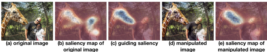
Figure 1: Example for saliency-guided image manipulation. The (b) saliency map of (a) original image indicates the human couple as the most salient object. Upon being conditioned on (c) the guiding saliency map which aims to attend more on giraffe, our proposed method edits the image accordingly to get (d) the manipulated output, with its corresponding saliency map shown in (e). Note here that we visualize the saliency map (which is single channel) by stacking it upon color images in order to provide their spatial correspondence.
