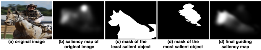
Figure 3: Example of generating guiding saliency map. The most salient object is changed from the rider to the horse.
