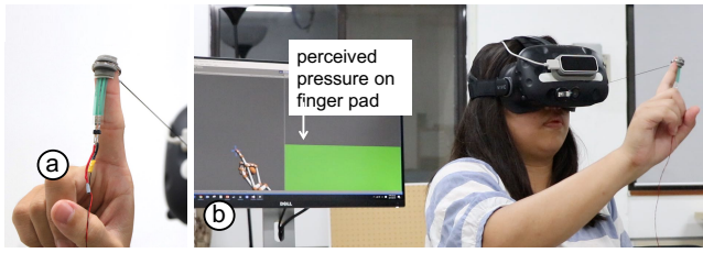
Figure 5: Experiment setup of Study 1. (a) A pressure sensor was placed between the pad and the user finger to record the perceived pressure. (b) Real-time display of pressure and tracking hand to ensure the detection was working well during study.
